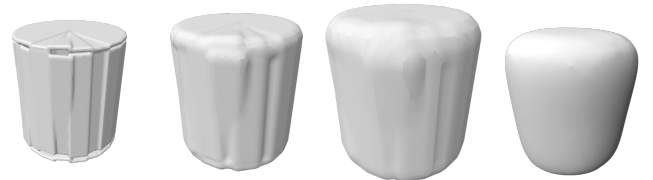
Fig. 4: We generated different mesh proxies for the triangle soup in Fig. 3. The first one fits the shape too closely to form a single mesh and cannot be used for a common parameterization of the triangle soup. The other mesh proxies have a larger offset parameter, what results in watertight meshes, which enclose the triangle soup. The rightmost mesh proxy was smoothed using Laplacian smoothing.
